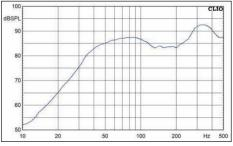
Musway MF108Q: With the MF108Q you can see a - Very Cleve hump between 200 and 300 Hz, which comes from the downfi re principle, this frequency range is of course affected by the Soft filtered away
