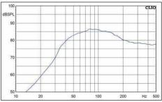
Musway MR206Q: The two 16s in the MR206Q ensure 86 dB characteristic sound pressure, the cut-off frequency of almost 50 Hz is fine for 15 liters
