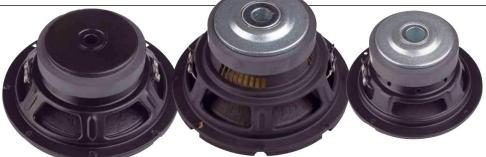
The MF woofer (left) is significantly flatter than the 20 in the MR108Q (middle). All woofers have solid sheet metal baskets and pressed pole cores, the 20s work with 2 x 2 ohm double voice coils
