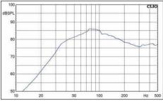
Musway MR108Q: The MR108Q is tuned to 46 Hz, with 85 dB at 1 W it is not too quiet for a 20
