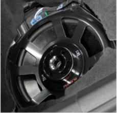
Now remove the original subwoofer, which is also attached with screws and disconnect the cable. Then replace subwoofer and reconnect the cable. Then install the cover of the subwoofer. Reinstall the seats and check that the screws are tight.
