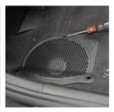
To install the subwoofer, the front seats must be removed, which are attached with 4 screws. After that, the accessible. Remove the subwoofer cover, which is attached with 4 screws.
