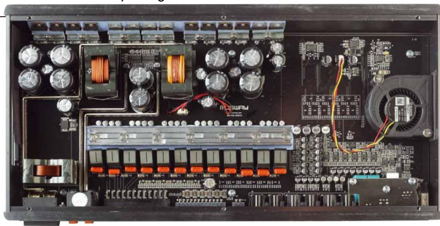
Clean construction with an extremely powerful double power supply with flat wire coils and a row of 12 low-pass coils under the narrow heat sink for the 6 amplifier ICs
